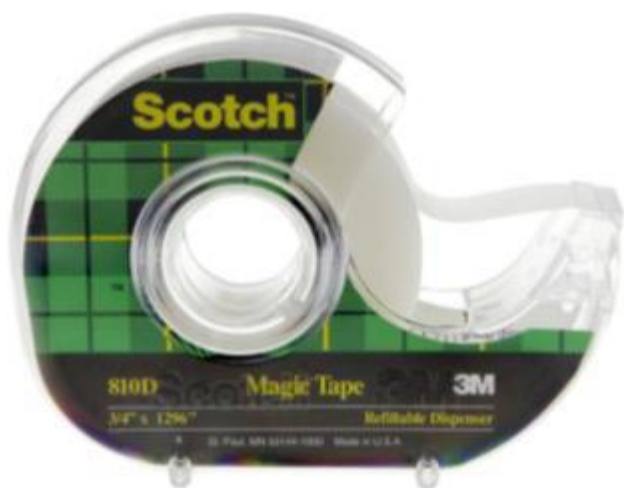
Figure 2.1: Scotch tape used for mechanical exfoliation [27]
