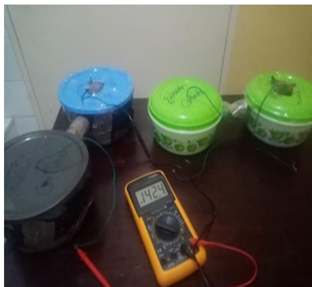
Figure 3: Double chamber microbial fuel cell setup and digital multimeter DT9205A-(Output readings).
