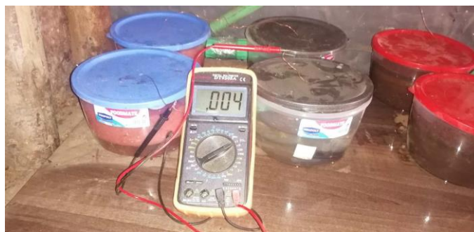
Figure 1 : Set-up of H-shaped microbial fuel cells with a multi-meter
