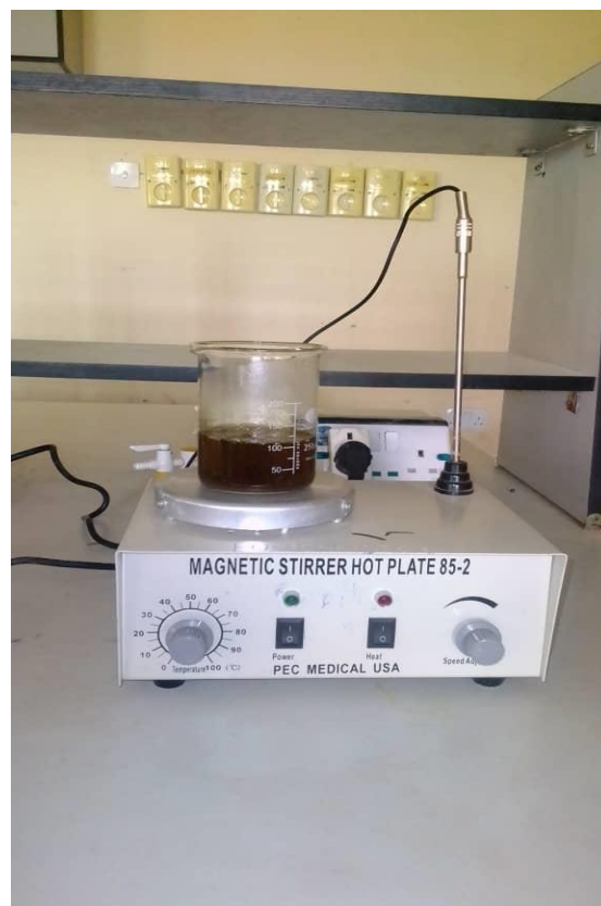
Figure 2:(a) Set up for Synthesis of AgNPs
